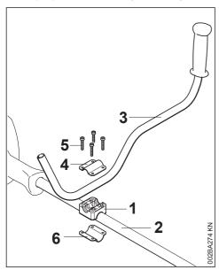
► Place the handle support (1) on the drive tube (2).
