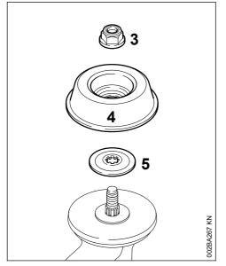
The nut (3), rider plate (4) and thrust washer (5) are required to secure some mowing heads.
