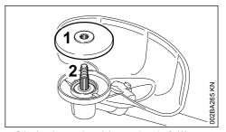
Slip the thrust plate (1) over the shaft (2).
