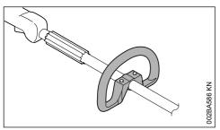
A factory-new machine comes with the loop handle already mounted.
