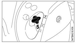
Press in the choke lever (5) and turn it to <u>T</u> at the same time.
