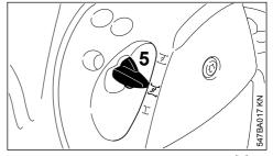
► Press in the choke lever (5) and turn it to <u>✓</u> at the same time.
