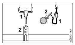
Attach the carabiner (1) to the carrying ring (2) on the drive tube
