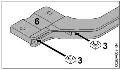
► Fit the square nuts (3) in the barrier bar (6); the holes must line up.
