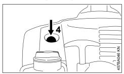
Press the manual fuel pump bulb (4) at least five times – even if the bulb is filled with fuel.
